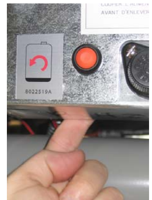
Figure 18: The electric reset switch is under the controller on the right side of the fryer.
